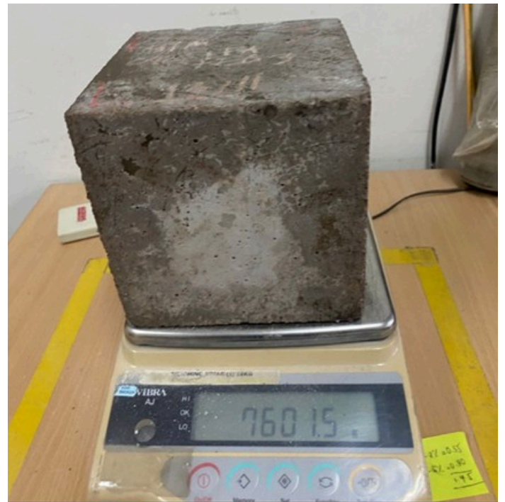
Figure 3: Weighing of saturated sample
