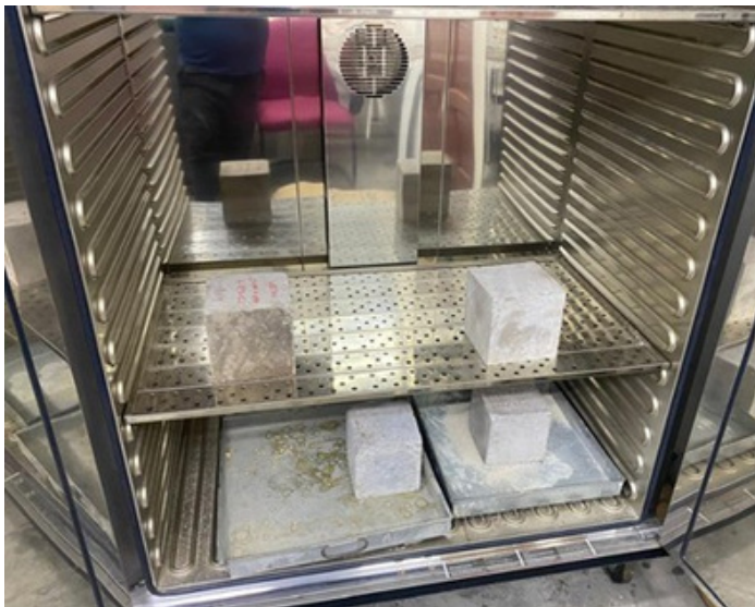
Figure 1: Drying hardened cubes in oven
