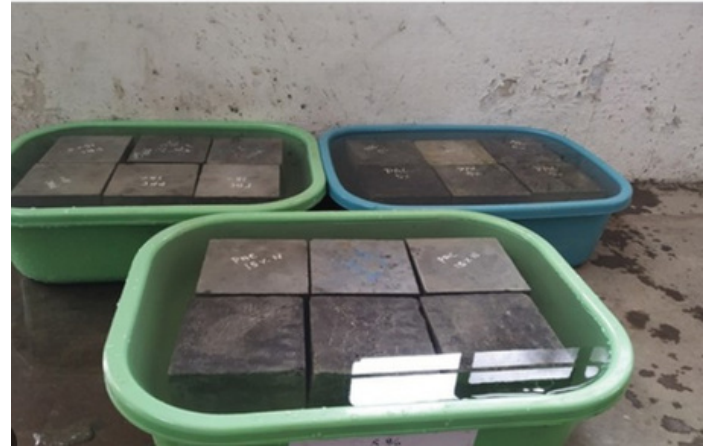
Figure 2: Submerged hardened concrete
